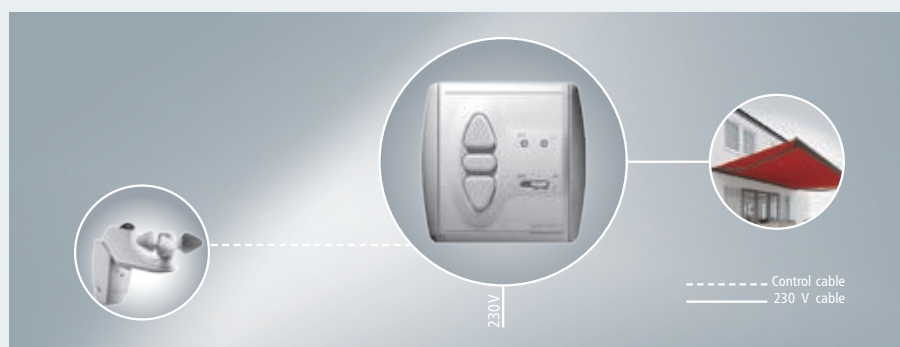
How the Uno cable system works
